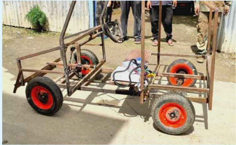
Prototype of an Electric Solar Vehicle (2020) designed and fabricated by Ginzalal, Laipubam Devshish Sharma, Monish Wakambam, and Wakambam Heera under the guidance of Haobam Jaillendro Khuman, Department of Electrical Engineering, Manipur Technical University.
